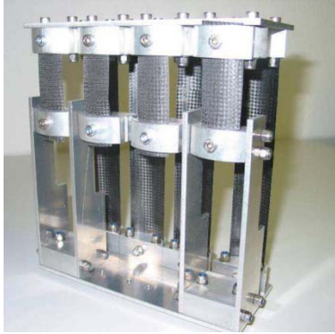
Self-motorized deployment mechanism Boesch et al. (2008)
